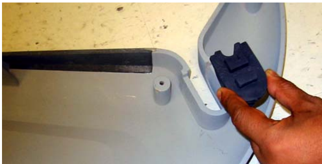
Figure 30. Installing a meter break cap in a plastic side cap
