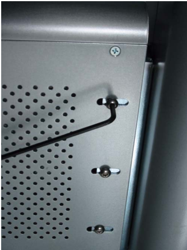
Figure 9. Attaching the crossbar
